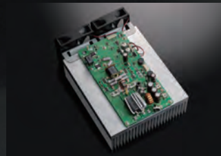
PA Unit with a Large Heatsink
